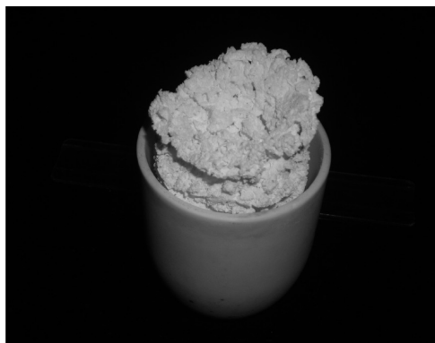
Figure 1. Voluminous \text{Li}_4\text{Ti}_5\text{O}_{12} formed after the combustion of corresponding metal nitrates with glycine at 800 °C.
